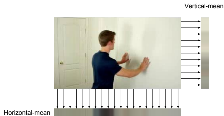
Figure 2.4: Modified spatio-temporal slice: the horizontal-mean/vertical-mean slice from a given frame contains the average of the columns/rows. The slices were resized for illustration purposes. Extracted from [17].
