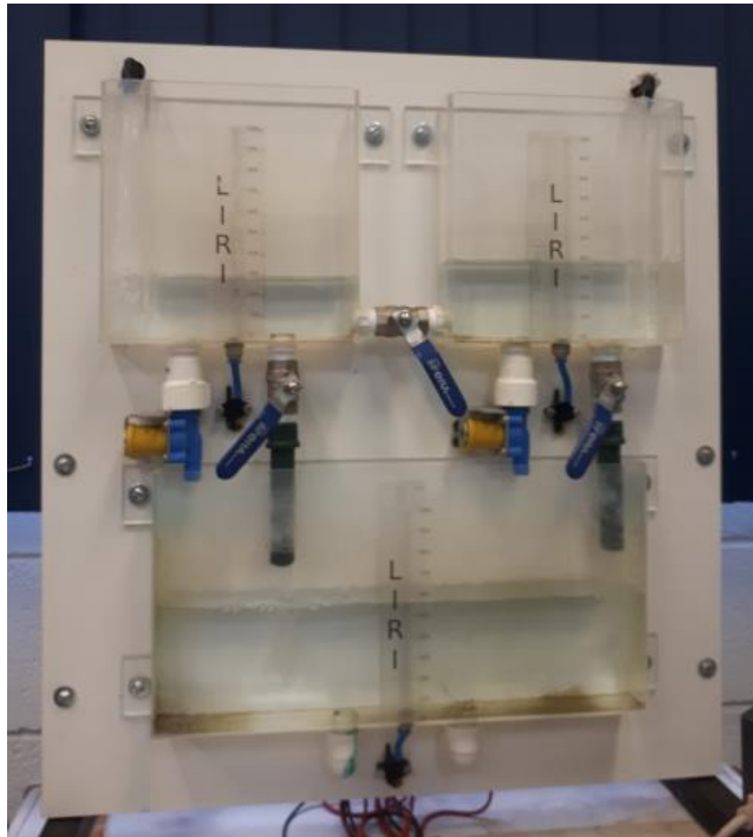
Figure 12: Experimental scheme of coupled tanks.
