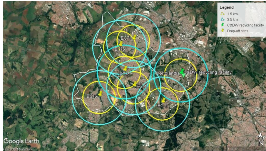
Figure 51. Coverage area of 1.5 km and 2.5 km of the sorting areas and C&DW recycling facility of the municipality of Hortolândia.
