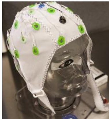
Figure 2.7. EEG positioning cap with gel based electrodes. Extracted from [Aalto university website].
