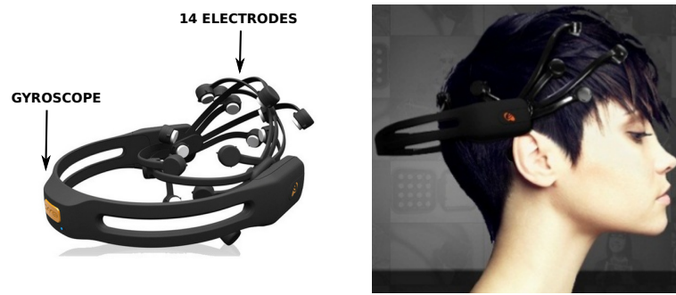
Figure 1 – Emotiv EPOC device with sensors to estimate the head orientation and detect facial expressions, thoughts and emotions. Adapted figure. 1
