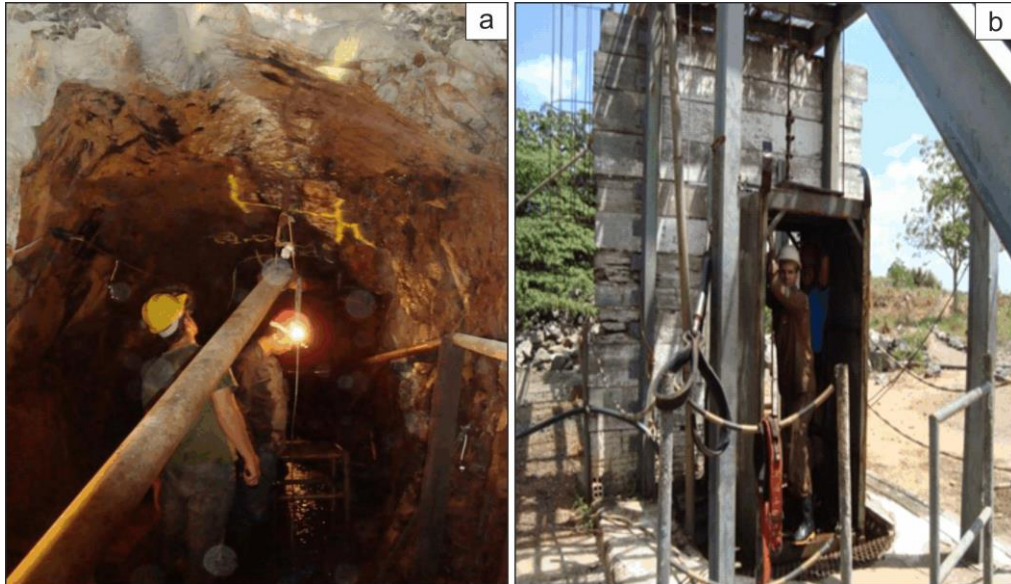
Figure 8: a) Gallery photograph, currently flooded. b) Location of the shaft and elevator for transporting material and workers during the operation time of the mine.
