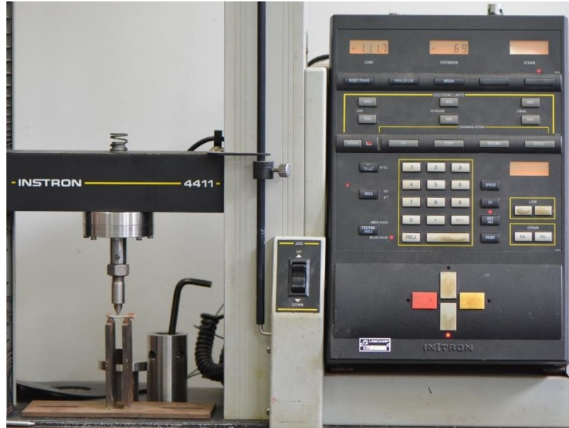
Figure 1. Three-point bending mechanical test on the Instron 4411 universal test machine.
