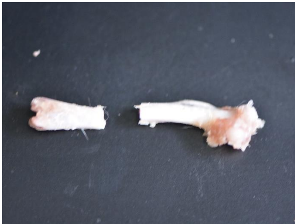
Figure 2. SHAM Femur, after the three-point bending test, showing a complete fracture.
