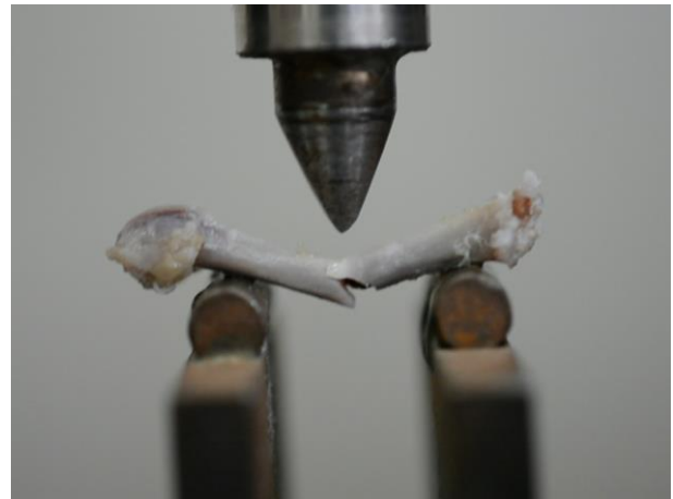
Figura 3. OVX femur after the three-point bending test, showing an incomplete fracture .
