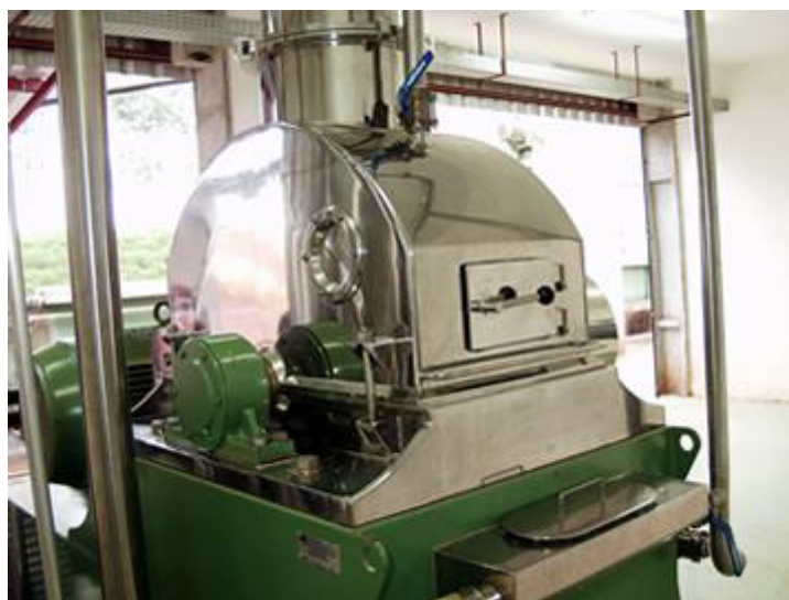
Figure 2.4: Cassava root industrial grater SOURCE: (EBS, 2017)
