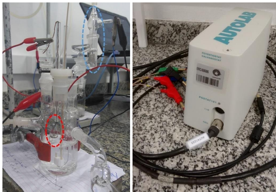
Figure 7: (left) electrochemical cell used on the electrochemical measurements, highlighting the working (red) and reference (blue) electrodes; (right) the potentiostat/galvanostat used to control the cell.
