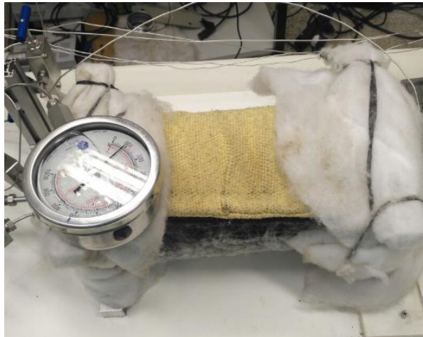
Figure 3.31 A resistance heating type jacket is wrapping around the core holder
