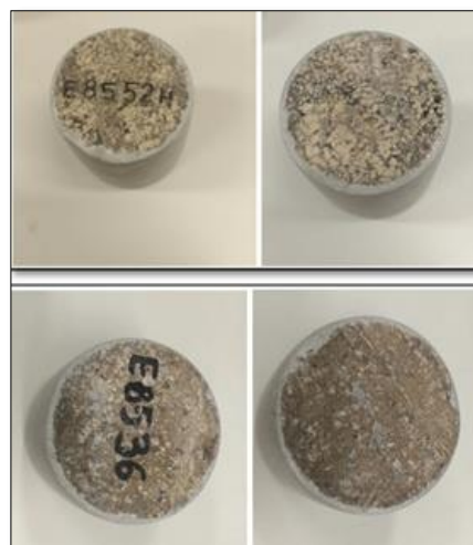
Figure 3.18 Cemented and sand down reservoir's rocks
