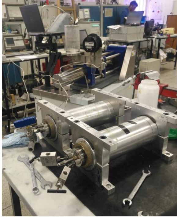
Figure 3.30 Introduced into overburden system until reached 1000 psi
