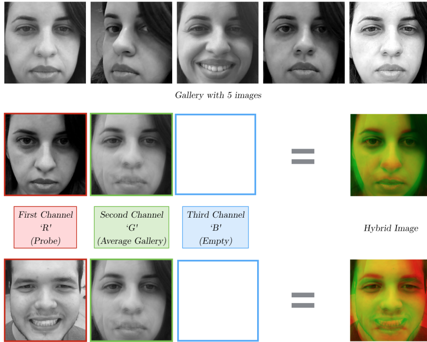
Figure 4.4: Generation of hybrid images, using a gallery with five images and two probes, one depicting the same identity as the gallery and another from a different person. The probe, the gallery average image and a zero image are stacked to compose the RGB hybrid image that is fed to the network. Our intuition is that the CNN is able to learn patterns that distinct same-identity hybrid images from different-identities ones.
