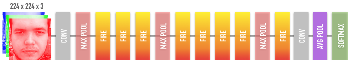
Figure 2.11: SqueezeNet architecture adapted from [40]. As we move forward in the network, the size of each Fire module (i.e., the number of filters in squeeze and expand layers) is gradually increased.
