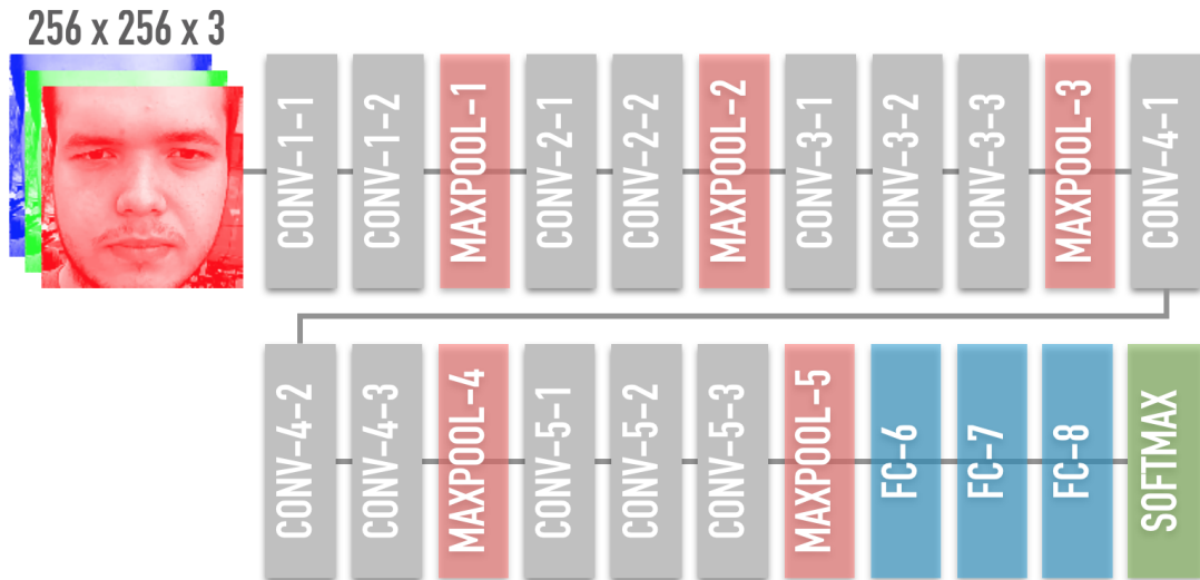
Figure 2.7: Representation of VGGNet architecture [64]. It receives a 256x256 RGB input image, has 13 convolutional layers (in grey) and 3 fully-connected layers (in blue). Detailed information about each layer, regarding its configuration, number of parameters and operations executed, is presented later in Table 4.1.
