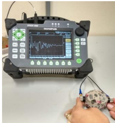
Figure 2. Ultrasound test on a polyhedral sample.
