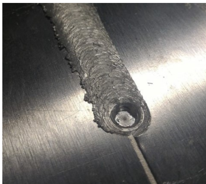
Figure 5.25: Probe exit of the weld of Case 3.
