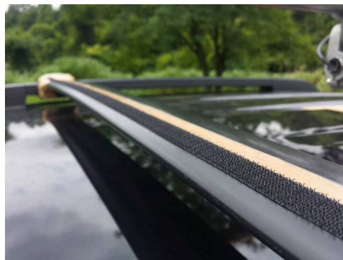
Figure 4.21: Turbulence Mesh Boundary Layer Tripping detail.
