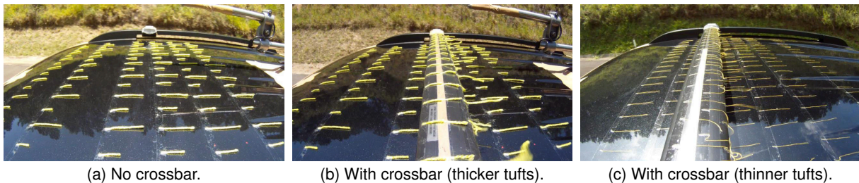
Figure 3.5: Roof flow visualization at 120km/h ( Re_c = 147,000 ).
