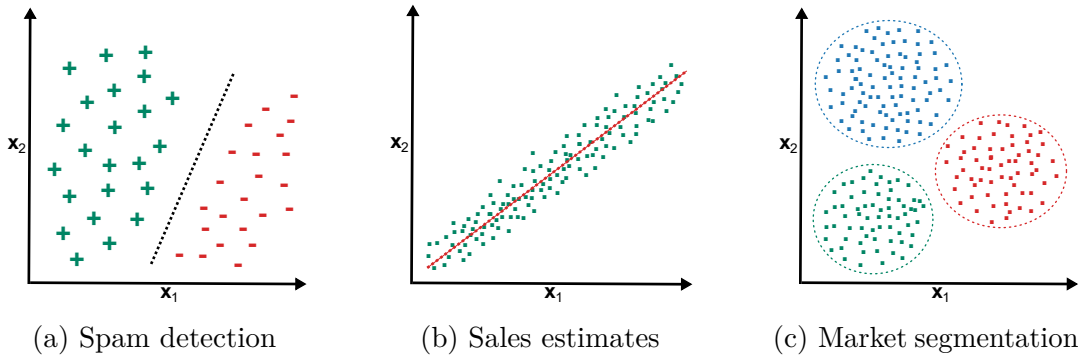
Figure 2.1 – Examples of learning tasks. (a) shows an example of a binary classification task, where the goal is to classify e-mails into spam or not spam. (b) shows an example of a linear regression task, where the goal is to predict sales for a determined store. (c) shows an example of a clustering task, where the goal is to identify customer groups potentially interested in the same market segment.
