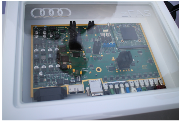
Figure 1.3 – Audi AG has chosen Austrian TTTech group to supply their zFAS system. The board uses a Cyclone™ V FPGA alongside a Tegra™ processor to capture and fuse data from various sensors. This data is used to provide ADAS services to the driver. The technology is present in the newer Audi A8 car.
