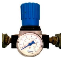
Figure 3. 3 - Photograph of the pressure regulator.
