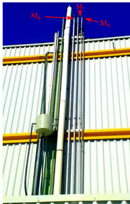
Figure 3. 8- Vertical production section with pressure transmitters M6, M7, M8
