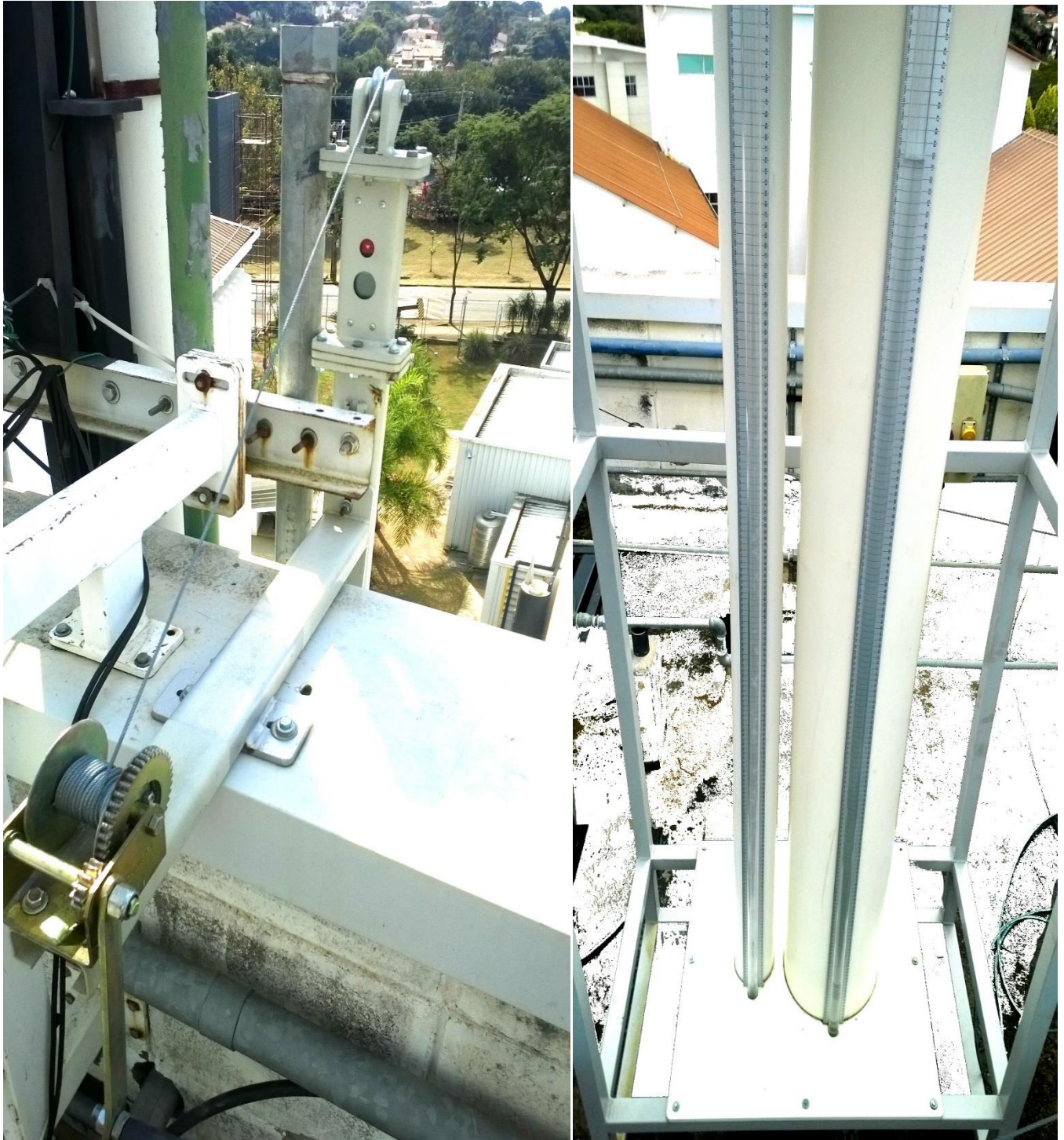
Figure A. 6– Photograph on the right portable tank elevation mechanism, on the left the separator
