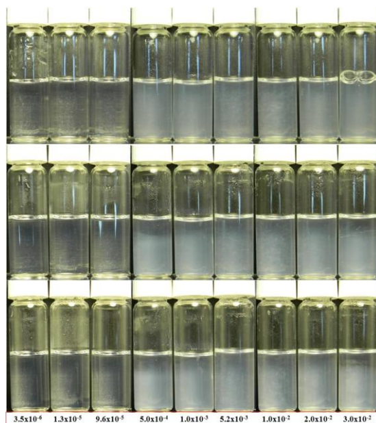
Figure A.8 Comparison of mixtures containing C_{16} TAB and 0.1 wt% CNC. The pictures were taken after preparation (top), after 1 week (middle), and after 2 months (bottom). The C_{16} TAB concentrations are expressed in \text{mol L}^{-1} .
