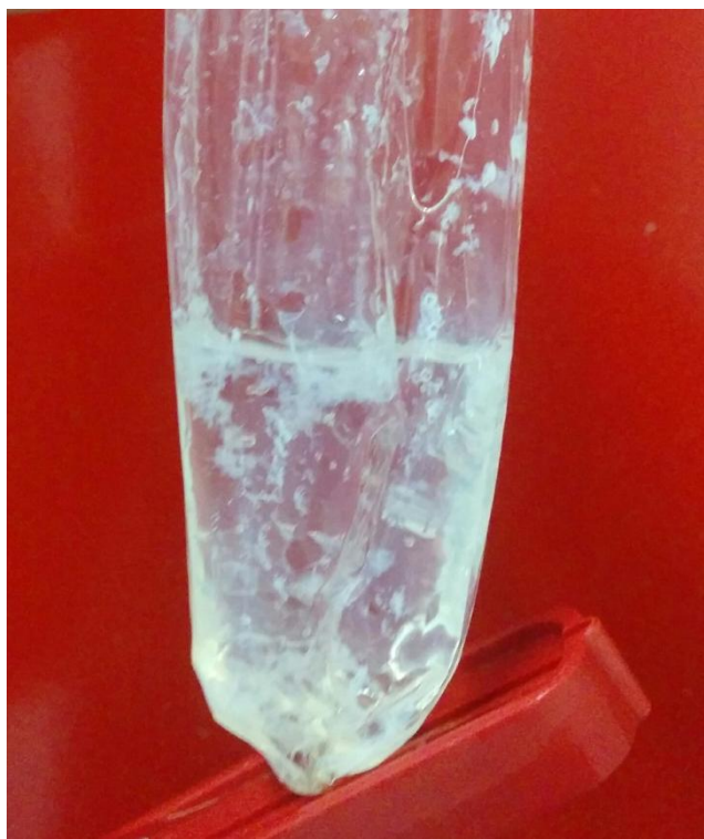
Figure B.7 Dialysis tube containing 1.0 wt% CNC-g-P(MEO 2 MA) and C 12 TAB 80.0 mmol kg -1 . Result obtained after 1week of dialysis, replacing the water three times a day.
