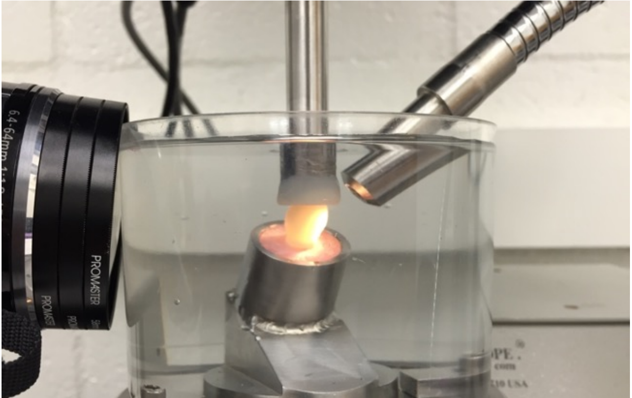
Fig. 3. Specimen in load chamber. Macro-camera and transillumination light was used to identify the crack propagation mode.
