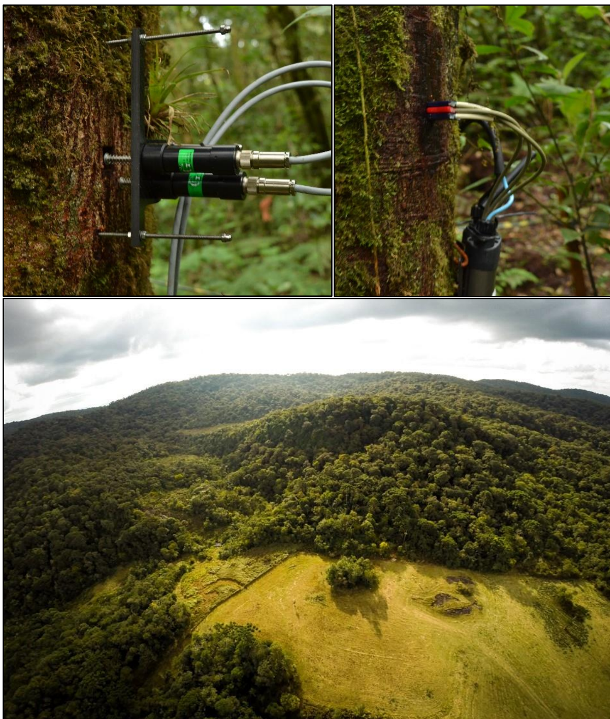
Figure 3. Upper left: High-resolution point dendrometer used to measure bark diameter changes. Upper right: Heat-ratio method sap flow sensor used to monitor tree sap velocity. Bottom: Aerial view of the tropical montane cloud forest fragment studied on this thesis. The fragment is located in Campos do Jordão, SP – Brazil at approximately 2000 m above sea level. Bottom picture by Vitor Barão.
