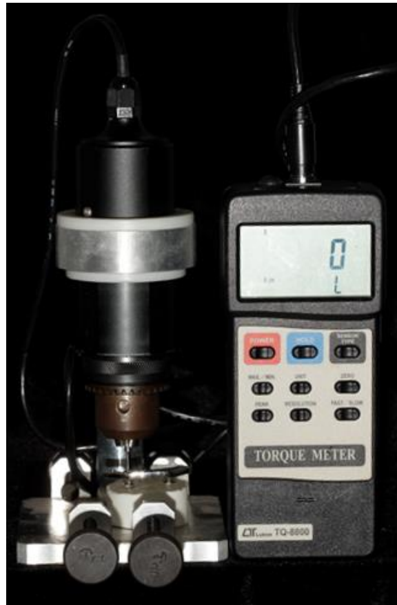
Figure 2 – Detorque reading with a torque meter
