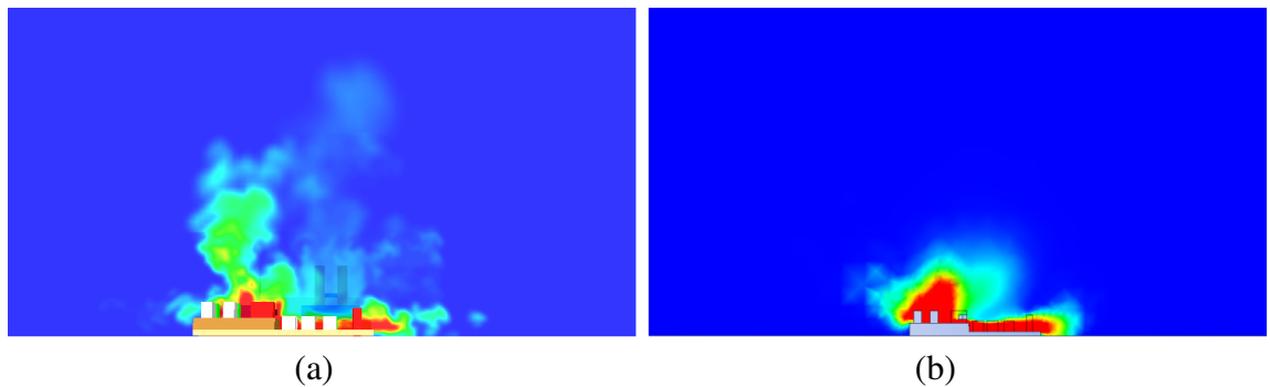
Figure 5.28: Front viewer screen shot of methane concentration dispersion transported by the wind blowing from the South. Slice at 18.5m perpendicular of x direction. (a) FDS code. (b) ANSYS-CFX code.
