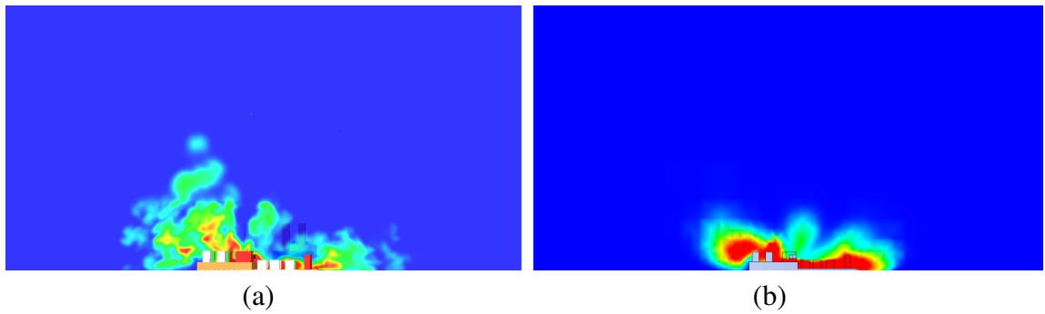
Figure 5.27: Front viewer screen shot of methane concentration dispersion transported by the wind blowing from the North. Slice at 18.5m perpendicular of x direction. (a) FDS code. (b) ANSYS-CFX code.
