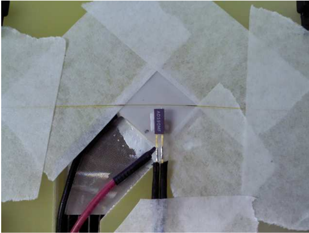
Figure C.8: Internal view of the thermal chamber, FBG installation.
