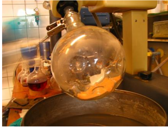
Figure I.7: Coated material after solubilizer evaporation (chromosorb + solvent).
