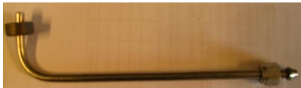
Figure I.4: 304 Stainless steel column.
