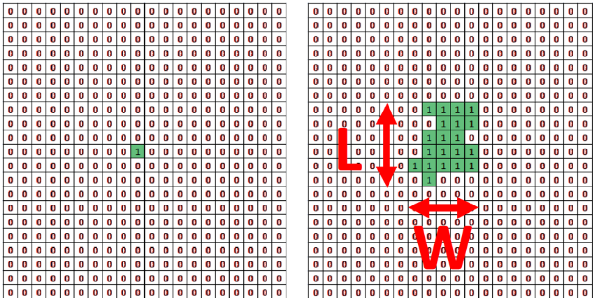
Figure B4c: (left) Initial M_{ij} matrix with a seed and (right) result after the iterative calculation until 20 neighbor blocks. The L and W refer to the maximum dimensions along i and j directions.
