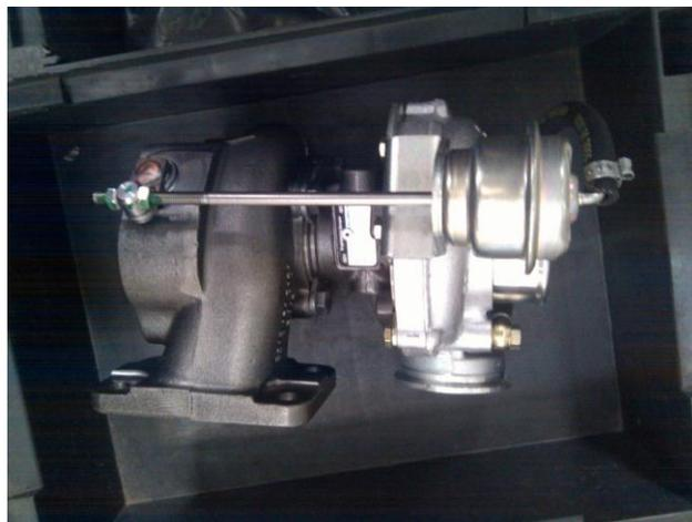
Figura 24: Turbocompressor BorgWarner
