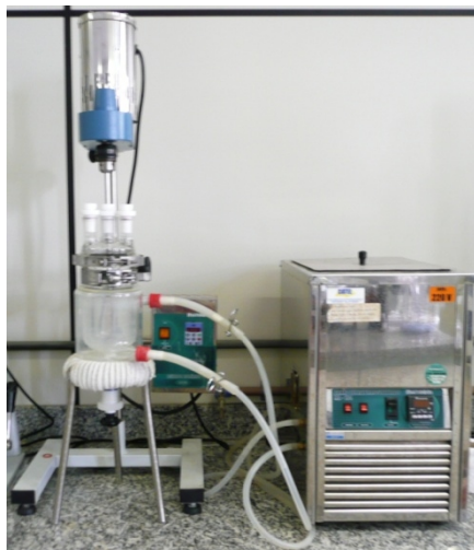
Figure 1. Experimental set-up for transesterification of castor oil
