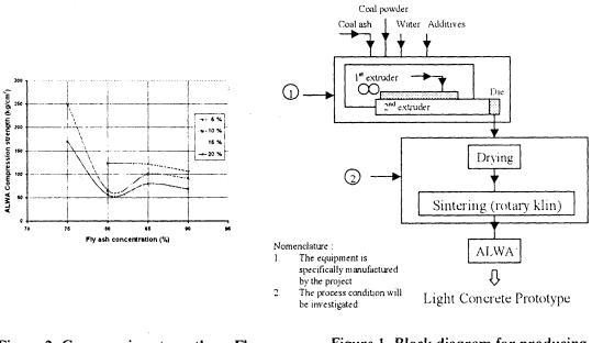
Figure 2. Compression strength vs. Fly Ash concentration
