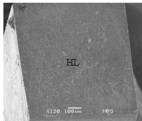
Figure 9. SEM observations of the fractured dentin surfaces. (a) Cohesive in bonding resin. (b) Mixed failure, at the hybrid layer, bonding resin and resin composite (c) Cohesive in hybrid layer. RC, resin composite; BR, bond resin; HL, hybrid layer.
