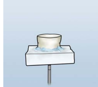
Fig. 3 Crown-segments glued to Plexiglass slabs.
