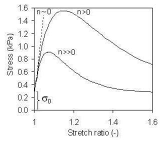
Figure 3. Schematic representation of Equation 3 for different values of n, n>0. The dashed line represents the ideal elastic behaviour obtained for very low n values  $(n\sim0)$ . The solid lines represent the behaviour for higher n values (n>0, n>>0).
