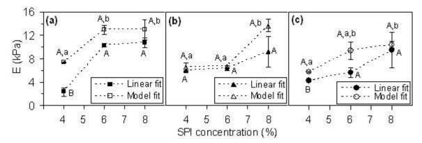
Figure 6. Variation of Young modulus (E) as a function of SPI concentration for GDL-induced gels: SPI at 25 °C (a), SPI + 0.2% xanthan at 25 °C (b), SPI + 0.2% xanthan at 10 °C (c). Different letters indicate significant differences at p<0.05 (small letters: variation of  $E_{model}$  with SPI concentration for each type of GDL-gel; capital letters: comparisson between  $E_{model}$  and  $E_{linear}$  for each concentration and GDL-gel type).
