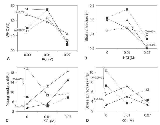
Figure 9. Variation in the water holding capacity (A), strain at fracture (B), Young modulus (C) and stress at fracture (D) at three KCl concentrations. X is the xanthan concentration: 0.05 wt% ( $\blacksquare$ ,  $\square$ ), 0.3 wt% ( $\blacktriangle$ ,  $\triangle$ ). SPI: 10 wt% ( $\blacksquare$ ,  $\blacktriangle$ ), 14 wt% ( $\square$ ,  $\triangle$ ).
