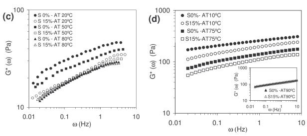
Figure 4. Temperature dependence of  $G^*(\omega)$  for different concentrations of the xanthan solutions at  $10^{\circ}$ C. The solutions were prepared at different annealing temperatures (AT) and added by 15% of sucrose (S). a) X01, b) X05, c) X1, d) X35.
