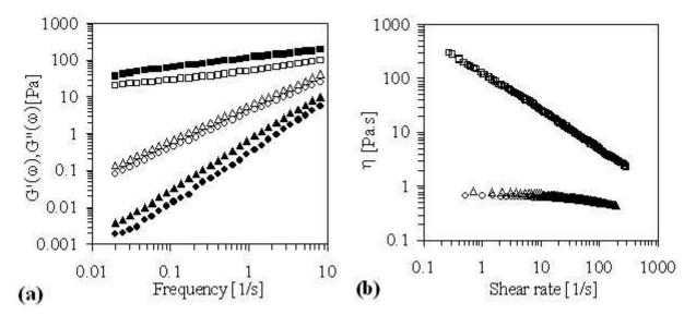
Figure 4. Frequency sweep (a) and flow curve (b) for  $SA_2$  system (SPI 3% – Na-alginate 2.5%) mixed solution ( $\blacktriangle$ ) and the rich protein ( $\blacksquare$ ) and polysaccharide ( $\bullet$ ) phases after centrifugation at 60000g for 1h. Closed symbols correspond to  $G'(\omega)$  and open symbols correspond to  $G''(\omega)$  or  $\eta$ .
