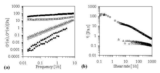
Figure 6. Frequency sweep (a) and flow curves (b) for  $SA_1$  system (SPI 3% – Na-alginate 1.5%), mixed solution ( $\blacktriangle$ ), protein ( $\blacksquare$ ) and polysaccharide ( $\bullet$ ) rich-phases after centrifugation at 60000g for 1h. Closed symbols correspond to  $G'(\omega)$  and open symbols correspond to  $G''(\omega)$  or  $\eta$ .
