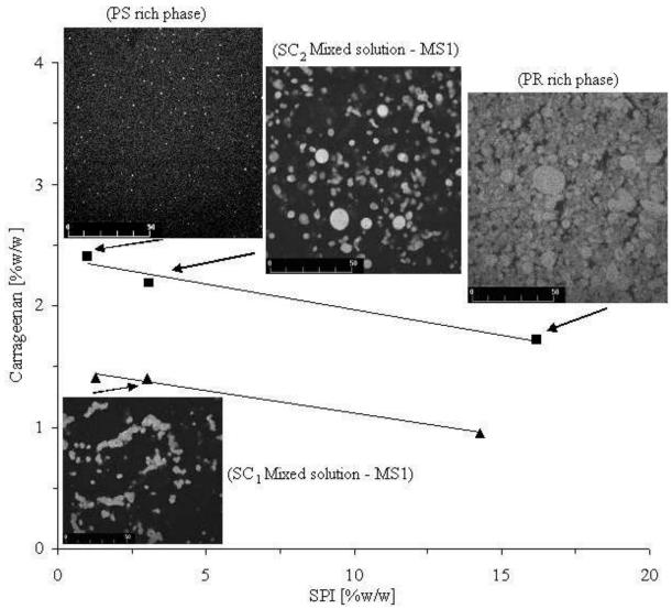
Figure 7. Confocal micrographs at 25  $^{\circ}$ C of the mixed solution, protein- and polysaccharide-rich phases of SC<sub>1</sub> and SC<sub>2</sub> (SPI – Carrageenan) systems. Closed symbols are experimentally determined biopolymer concentrations of MS, PR<sub>rp</sub> and PS<sub>rp</sub>. The light regions in the micrographs indicate protein area, scale bar =  $50\mu m$ .
