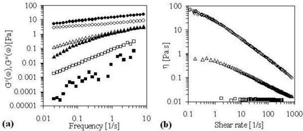
Figure 13. Frequency sweeps (a) and flow curves (b) for CG (Na-caseinate 5% – gellan 0.4%) mixture ( $\blacktriangle$ ), protein ( $\blacksquare$ ) and polysaccharide ( $\bullet$ ) rich-phases after centrifugation at 60000g for 1h. Closed symbols correspond to  $G'(\omega)$  and open symbols correspond to  $G''(\omega)$  or  $\eta$ .
