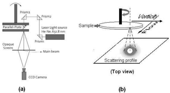
Figure 2. Schematic of rheo-small angle light scattering constructed for the stress controlled Rheometrics<sup>®</sup> DSR rheometer (a) and the top view of a typical scattering profile (b).
