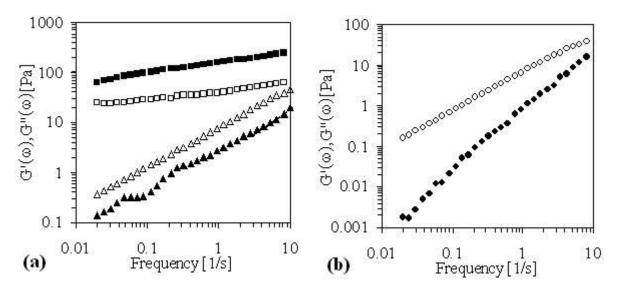
Figure 17. Frequency sweeps for CC (Na-caseinate – carrageenan). A) Mixture ( $\blacktriangle$ ) and the protein rich phase ( $\blacksquare$ ), B) polysaccharide rich phase ( $\bullet$ ). Closed symbols correspond to G'( $\omega$ ) and open symbols correspond to G''( $\omega$ ).
