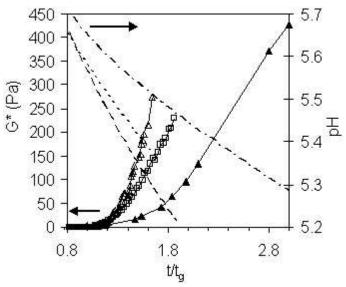
Figure 2. Complex modulus ( $G^*$ ) and pH evolution during the acidification of SPI solutions as a function of the reduced time ( $t/t_g$ ). Systems: 4% SPI-  $G^*$  ( $\square$ ), pH (dashed line); 8% SPI-  $G^*$  ( $\Delta$ ), pH (dotted line); 8% SPI + 0.2% xanthan-  $G^*$  ( $\triangle$ ), pH (dot/dashed line).
