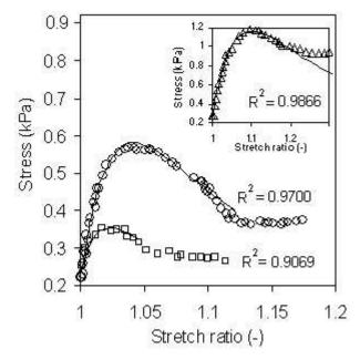
Figure 4. Stress-stretch profile of GDL-SPI gels at 25 °C. Systems: 4% SPI ( $\square$ ), 6% SPI ( $\square$ ), 8% SPI ( $\Delta$ ). The lines represent fits according to the model of Equation 3.
