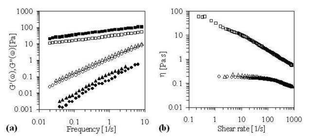
Figure 8. Frequency sweeps (a) and flow curves (b) for  $SC_1$ -system (SPI 3% – carrageenan 1.4%) mixture ( $\blacktriangle$ ), protein ( $\blacksquare$ ) and polysaccharide ( $\bullet$ ) rich-phases after centrifugation at 60000g for 1h. Closed symbols correspond to  $G'(\omega)$  and open symbols correspond to  $G''(\omega)$  or  $\eta$ .
