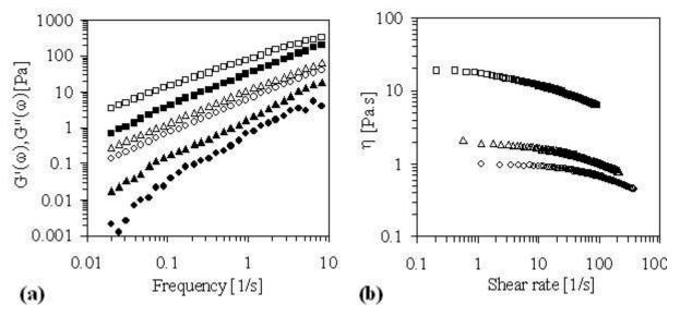
Figure 15. Frequency sweeps (a) and flow curves (b) for CA (Na-caseinate 2.9 % – Na-alginate 2.3 %) mixture ( $\blacktriangle$ ), protein ( $\blacksquare$ ) and polysaccharide ( $\bullet$ ) rich-phases after centrifugation at 60000g for 1h. Closed symbols correspond to  $G'(\omega)$  and open symbols correspond to  $G''(\omega)$  or  $\eta$ .
