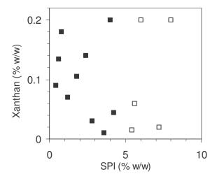
Figure 2. Compatible, one-phase, ( $\blacksquare$ ) and incompatible, two-phases ( $\square$ ) regions of SPI-xanthan mixtures, pH 7.0.
