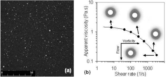
Figure 6. Rheological and optical characterization of the MS2 system (1%  $PR_{rp}$  + 99%  $PS_{rp}$ ) containing 0.4% Na-caseinate and 2.5%  $\kappa$ -carrageenan. A) Confocal microstructure; B) Apparent
