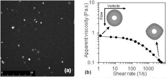
Figure 5. Rheological and optical characterization of the MS2 system (1%  $PR_{rp}$  + 99%  $PS_{rp}$ ) containing 1.2% SPI and 2.4%  $\kappa$ -carrageenan. A) Confocal microstructure; B) Apparent viscosity and 2D-SALS pattern as a function of the shear rate, the line represent the fit of Cross equation to the data. The light regions in the CLSM micrograph (a) indicate protein area, scale bar = 50 $\mu$ m.
