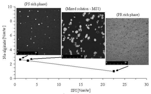
Figure 3. Confocal micrographs at 25  $^{\circ}$ C of the mixed solution, protein and polysaccharide rich phases of SA<sub>2</sub> (SPI - Na-alginate) system. Squares are experimentally determined biopolymer concentrations of MS, PR<sub>rp</sub> and PS<sub>rp</sub>. The light regions in the micrographs indicate protein area, scale bar =  $50\mu m$ .
