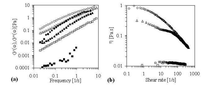
Figure 11. Frequency sweeps (a) and flow curves (b) for SG (SPI 4.8% - Gellan 0.4%) mixture ( $\blacktriangle$ ), protein ( $\blacksquare$ ) and polysaccharide ( $\bullet$ ) rich-phases after centrifugation at 60000g for 1h. Closed symbols correspond to G'( $\omega$ ) and open symbols correspond to G''( $\omega$ ) or  $\eta$ .
