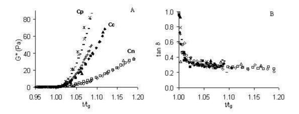
Figure 1. Rheological properties of acidified sodium-caseinate solutions as a function of the reduced time,  $t/t_g$ . A) Complex modulus (G\*) B) Loss tangent (tan  $\delta$ ). The oscillatory tests were done at 10°C and 0.1 Hz for solutions with different GDL/caseinate ratios for each sodium-caseinate content (Cp = 6%, Cc = 4%, Cn = 2%).
