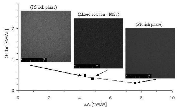
Figure 10. Confocal micrographs at 25  $^{\circ}$ C of the mixed solution, protein and polysaccharide rich phases of SG (SPI - Gellan) system. Squares are experimentally determined biopolymer concentration of MS,  $PR_{rp}$  and  $PS_{rp}$ . The light regions in the micrographs indicate protein area, scale bar =  $50\mu m$ .
