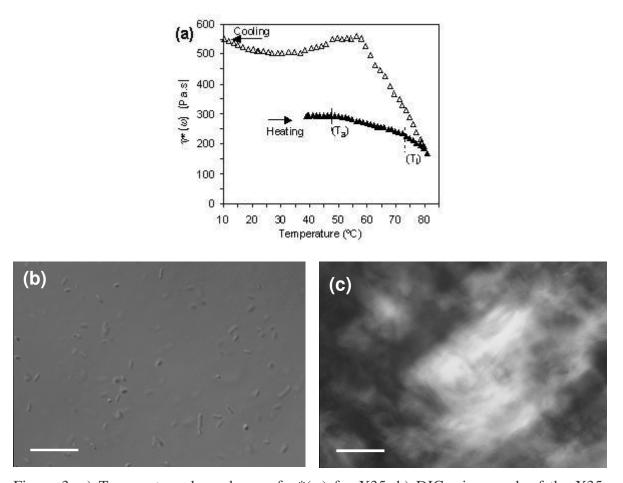
Figure 3. a) Temperature dependence of  $\eta^*(\omega)$  for X35. b) DIC micrograph of the X35 sample at 25°C. c) Polarized (PL) micrographs of the X35 sample at 25°C. Scale bars = 50  $\mu$ m.
