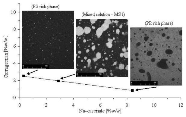
Figure 16. Confocal micrographs at  $25^{\circ}$ C of the mixed solution, protein and polysaccharide rich phases of CC (Na-caseinate –  $\kappa$ -carrageenan) system. Squares are experimentally determined biopolymer concentrations of MS,  $PR_{rp}$  and  $PS_{rp}$ . The light regions in the micrographs indicate protein area, scale bar =  $50\mu m$ .
