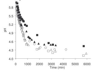
Figure 2. Changes in the pH of sodium-caseinate solutions during acidification with different concentrations of GDL. Formulations: ( $\blacksquare$ ) CnGn, ( $\square$ ) CnGp, ( $\bigcirc$ ) CcGc, ( $\blacktriangle$ ) CpGn, ( $\triangle$ ) CpGp.
