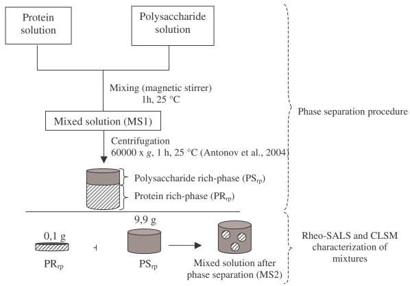
Figure 1. Procedure to prepare the protein-polysaccharide mixtures.
