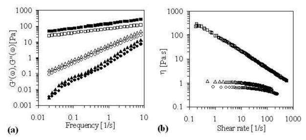
Figure 9. Frequency sweeps (a) and flow curves (b) for  $SC_2$ -system (SPI 3.1% – carrageenan 2.2%) mixture ( $\blacktriangle$ ), protein ( $\blacksquare$ ) and polysaccharide ( $\bullet$ ) rich-phases after centrifuging at 60000g for 1h. Closed symbols correspond to  $G'(\omega)$  and open symbols correspond to  $G''(\omega)$  or  $\eta$ .
