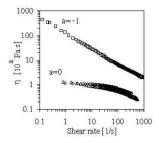
Figure 18. Flow curves for CC (Na-caseinate – carrageenan) mixture ( $\Delta$ ), protein ( $\square$ ) and polysaccharide ( $\bigcirc$ ) rich-phases after centrifugation at 60000g for 1h.
