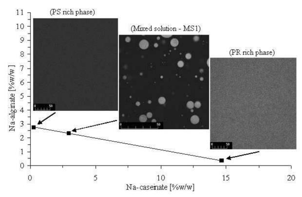
Figure 14. Confocal micrographs at  $25^{\circ}$ C of the mixed solution, protein and polysaccharide rich phases of CA (Na-caseinte – Na-alginate) system. Squares are experimentally determined biopolymer concentration of MS,  $PR_{rp}$  and  $PS_{rp}$ . The light regions in the micrographs indicate protein area, scale bar =  $50\mu m$ .
