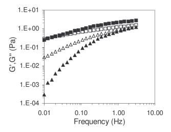
Figure 2. Frequency dependence of G' (solid symbols) and G" (open symbols) at 10°C for xanthan solutions prepared at 80°C with different ways of preparation: 3% with subsequent dilution to 0.3% or X-1 (squares); and 0.3% or X-2 (triangles).
