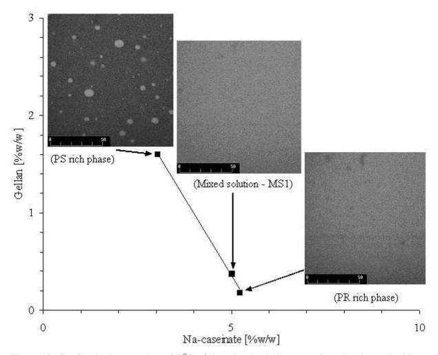
Figure 12. Confocal micrographs at 25  $^{\circ}$ C of the mixed solution, protein and polysaccharide rich phases of CG (Na-caseinte - Gellan) system. Squares are experimentally determined biopolymer concentration of MS,  $PR_{rp}$  and  $PS_{rp}$ . The light regions in the micrographs indicate protein area, scale bar =  $50\mu m$ .
