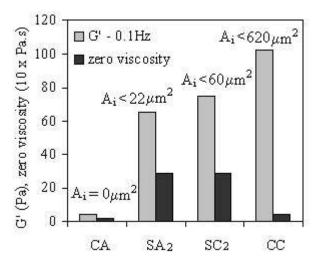
Figure 20. Rheological and morphological properties for the PR<sub>rp</sub> of different systems.
