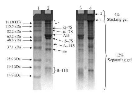
Figure 6. SDS-PAGE under non-reducing conditions: Lane 1 = molecular weight markers; Lane 2 = SPI powder; Lane 3 = soluble proteins of SPI gels extracted with deionized water; and Lane 4 = soluble proteins of SPI gels extracted with buffer (pH 8.0) plus urea. \*aggregates with MW higher than 115.5 kDa; \*\*low MW fractions.
