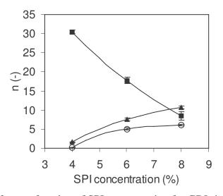
Figure 5. Variation of n as a function of SPI concentration for GDL-induced gels: SPI at 25  $^{\circ}$ C ( $\blacksquare$ ), SPI + 0.2% xanthan at 25  $^{\circ}$ C ( $\blacktriangle$ ), SPI + 0.2% xanthan at 10  $^{\circ}$ C ( $\bigcirc$ ). The solid lines represent the exponential fit to n values.
