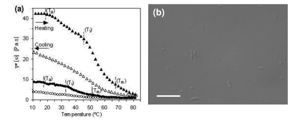
Figure 2. a) Temperature dependence of  $\eta^*(\omega)$  for X05 ( $\bullet$ ) and X1 ( $\blacktriangle$ ) on heating (closed symbols) and cooling (open symbols). b) DIC micrograph of the X1 sample at 25°C. Scale bar = 50  $\mu$ m.
