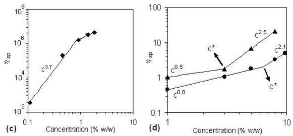
Figure 3. Concentration dependence of specific viscosity  $\eta_{sp}$  for polysaccharides and proteins. a)Na-alginate ( $\triangle$ ),  $\kappa$ -carrageenan ( $\blacksquare$ ); b LBG ( $\diamondsuit$ ), gellan ( $\bigcirc$ ); c) xanthan ( $\spadesuit$ ); d) SPI ( $\blacksquare$ ), Na-caseinate ( $\blacktriangle$ ). The long dashed line (b) represents the power law found by Richardson et al. (1981) for LBG.
