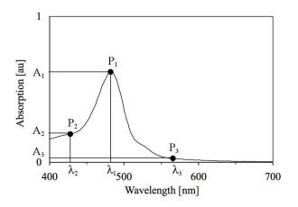
Figure 1. Typical light absorption curve of a polysaccharide solution with the description of the wavelengths used for the polysaccharide quantification.
