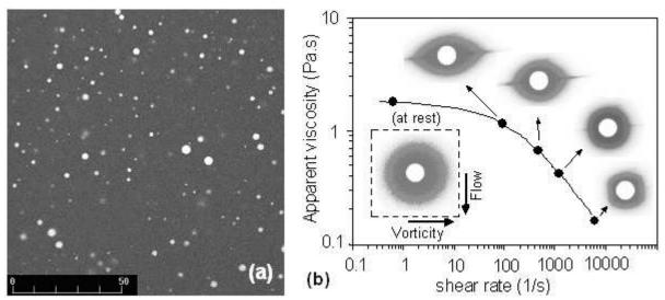
Figure 3. Rheological and optical characterization of the MS2 system (1%  $PR_{rp}$  + 99%  $PS_{rp}$ ) containing 0.44% Na-caseinate and 2.68% Na-alginate. A) Confocal microstructure; B) Apparent viscosity and 2D-SALS pattern as a function of the shear rate, the line represent the fit of Cross equation to the data. The light regions in the CLSM micrograph (a) indicate protein area, scale bar = 50 $\mu$ m.
