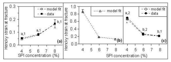
Figure 8. Variation of Hencky strain at fracture as a function of SPI concentration for GDL-induced gels: SPI at 25°C (a), SPI + 0.2% xanthan at 25°C (b), SPI + 0.2% xanthan at 10°C (c). Different letters and numbers indicate significant differences at p<0.05 (letters: variation of the property with SPI concentration for each type of GDL-gel; numbers: variation of the property with type of GDL-gel for each SPI concentration). \* Value divided by 15.
