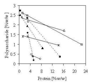
Figure 22. Phase composition for different protein-polysaccharide mixtures. CG ( $\bullet$ ), CA ( $\blacksquare$ ), CC ( $\blacktriangle$ ), SG ( $\bigcirc$ ), SA<sub>2</sub> ( $\square$ ), SC<sub>2</sub> ( $\triangle$ ),SC<sub>1</sub> (\*). Continuous line is the tie-line for SPI systems, dashed line is the tie-line for Na-caseinate systems.
