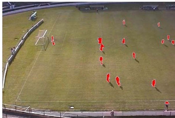
Fig. 3.23: Elimination of shadows by simple morphological operations.
