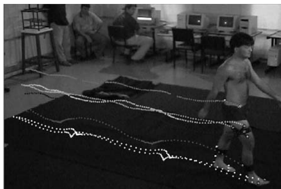
Fig. 2.13: One camera view tracking of reflexive markers applied for gait analysis.
