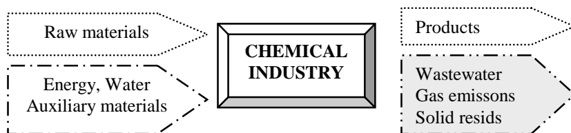
Figure 1. Typical flow scheme of a chemical industry.
