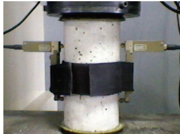
Figure 1. Position of clip-on strain gauges on the CS for the concrete modulus of the elasticity test.
