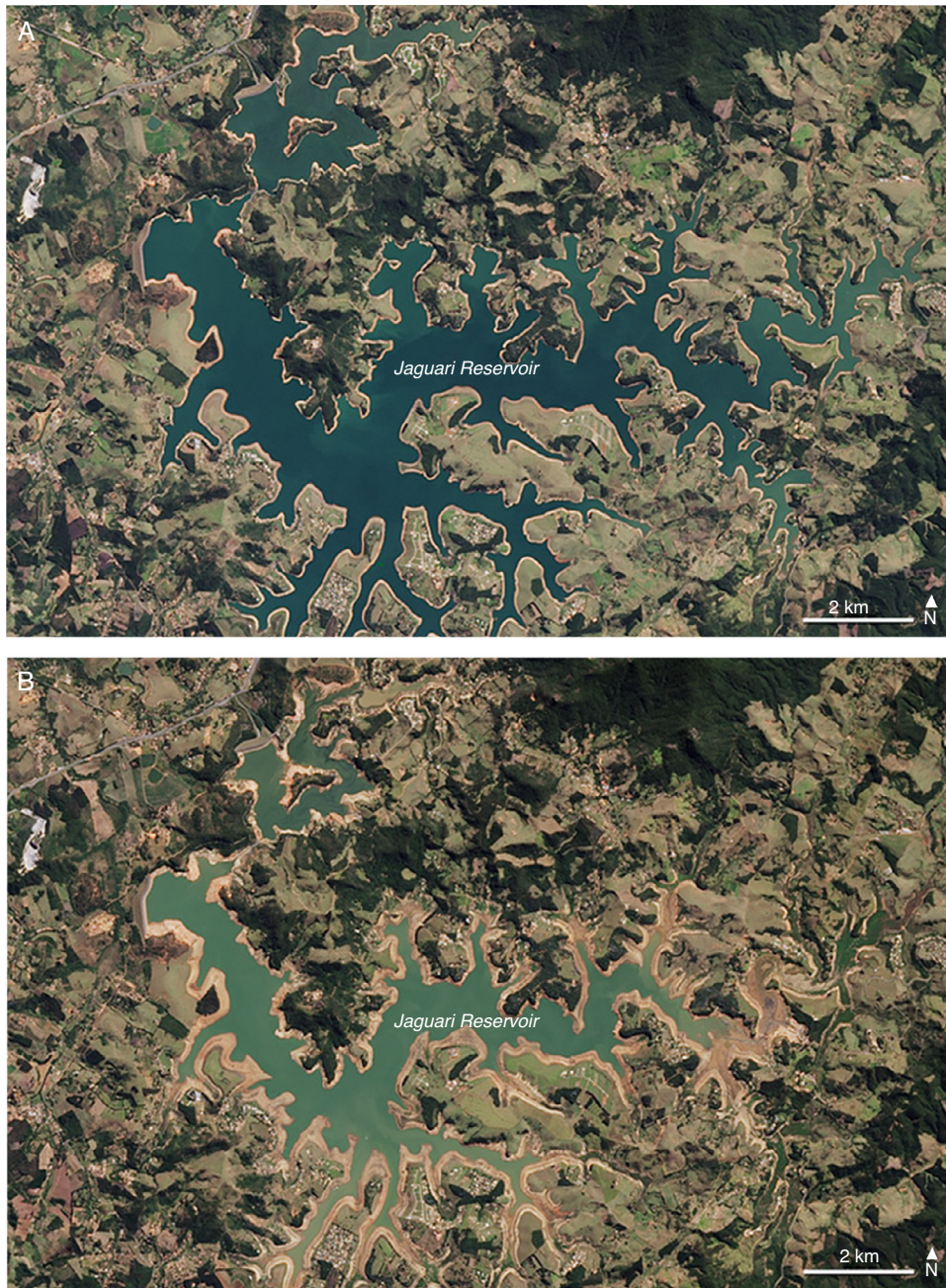
Fig. 1 – View of the Jaguari reservoir, which is part of the Cantareira system in August, 2013 (A) and August, 2014 (B). The level of lake is lower during the drought of 2014 as shown by the smaller area and by the lighter blue-green color of water. Notice the reduced forest cover in the area, including the margins of the reservoir. Images from NASA Earth Observatory.
