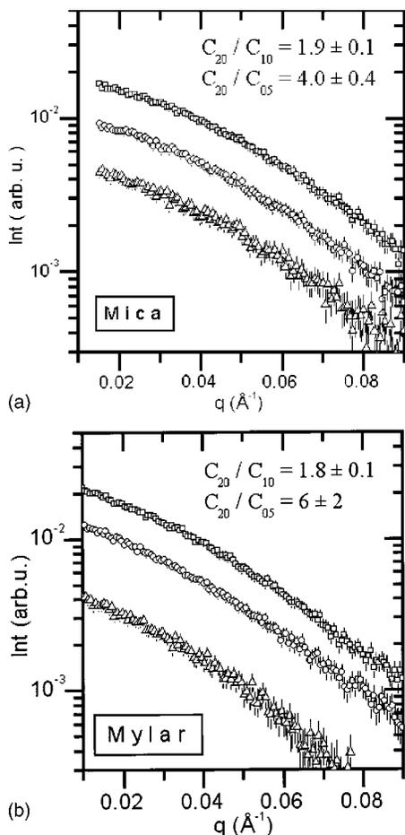
FIG. 4. SAXS intensity curves from three different concentrations of albumin in buffer solution for (a) Mica cell and (b) Mylar cell. □ 20, ○ 10, and △ 5 mg/ml. Intensity ratios should match concentration ratios. A good approximation to the 4:2:1 ratios is found for the mica cell.
