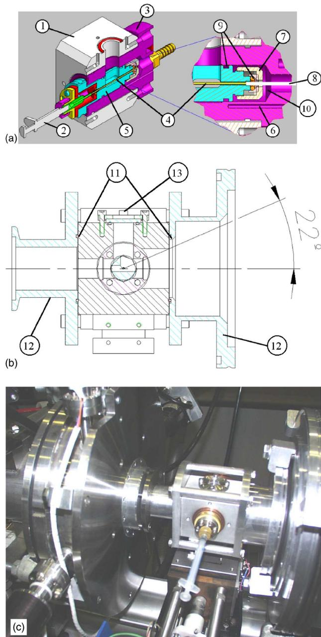
FIG. 2. (Color online) (a) Section view of the capillary cell chamber: (1) aluminum block, (2) syringe, (3) hollow copper shell, (4) capillary, (5) brass cylindrical core cell, (6) thermocouple path, (7) conical Teflon cap, (8) silicon tube, (9) O-rings, and (10) metal cap. (b) Details of the sample cell: (11) O-rings, (12) flanges, and (13) view port. (c) Complete sample holder installed at the SAXS beamline of the LNLS.
