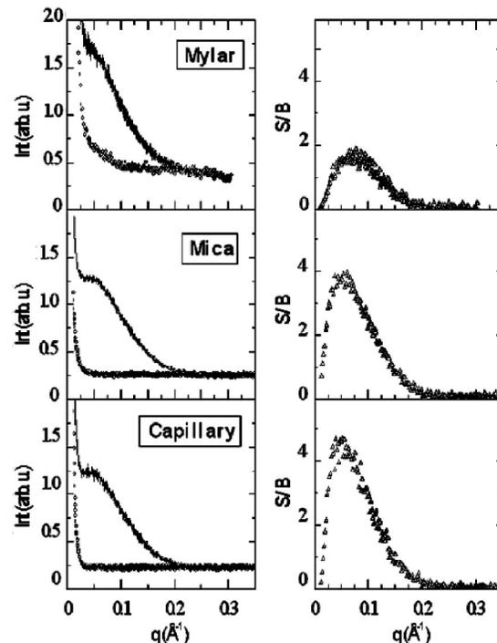
FIG. 3. Measured scattering intensity from a Lysozyme buffer solution (20 mg/ml) (full line) and from the buffer solution (open circles). The signal-to-background S/B ratio ( $= [I_{\text{Lys}} - I_{\text{Buf}}] / I_{\text{Buf}}$ ) is plotted for each sample holder: (a) disposable Mylar cell, (b) mica cell, and (c) capillary cell.
