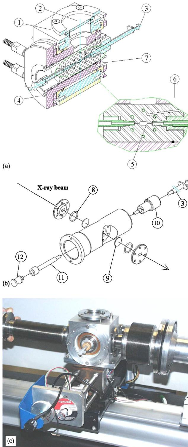
FIG. 1. (Color online) (a) Section view of the mica cell chamber: (1) aluminum block, (2) view port, (3) syringe, (4) hollow copper shell, (5) sample space, (6) thermocouple path; and (7) O-rings. (b) Details of the stainless steel sample cell: (8) O-ring, (9) mica windows, (10) Teflon adapter for syringe, (11) Teflon connector for drain hose or sealing cap, and (12) sealing cap. (c) Photograph of the sample holder installed at the SAXS beamline of the LNLS.
