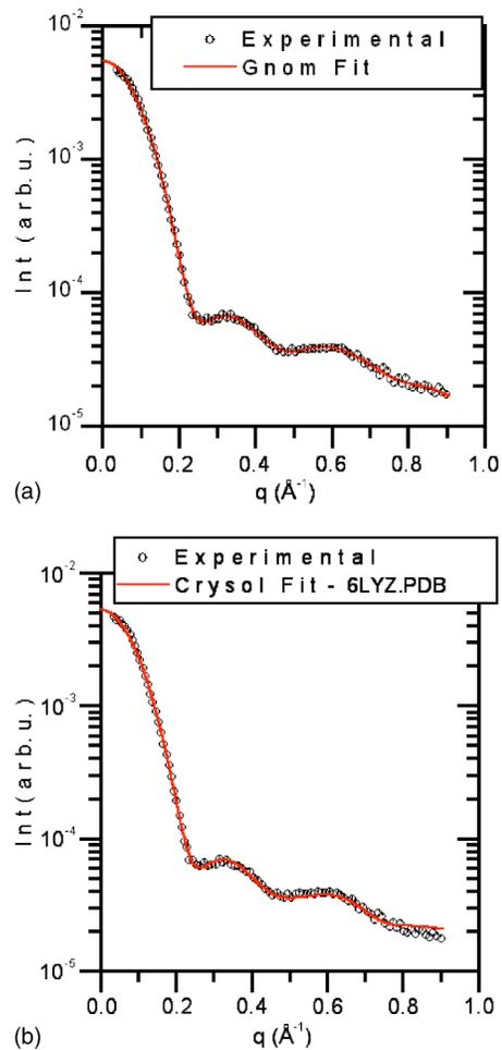
FIG. 5. (Color online) (a) One dimensional scattering curve obtained by radial integration of 2D scattering data from a Lysozyme buffer solution. The experimental points have been fitted using the GNOM program. (b) Comparison of the experimental data and the calculated scattering curve obtained from the crystallographic coordinates (6LYZ.pdb) using the CRY SOL program.
