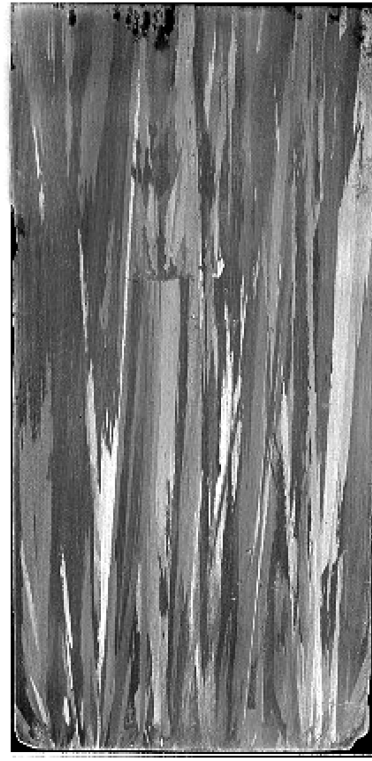
Fig. 8—Macrostructures: (a) Al 2 wt pct Cu, coated mold, and T_p = 689^\circ\text{C} ; (b) Al 5 wt pct Cu, polished mold, and T_p = 680^\circ\text{C} ; (c) Al 8 wt pct Cu, polished mold, and T_p = 690^\circ\text{C} ; (d) Al 10 wt pct Cu, coated mold, and T_p = 705^\circ\text{C} ; (e) Sn 10 wt pct Pb, coated mold, and T_p = 220^\circ\text{C} .
