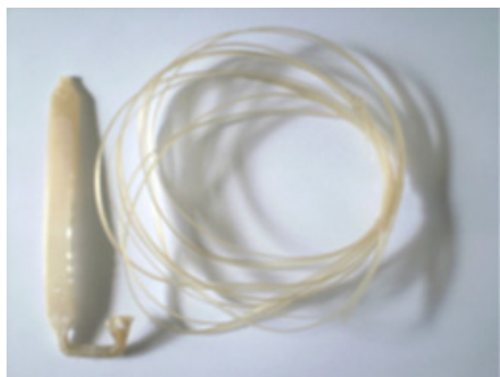
Figure 2: Example of a sample of nanocomposite prepared in the microextruder (Nano_Vulgel O2).
