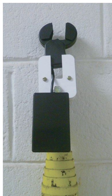
Fig.6 The mini-clamp meter ready to be installed, in the tip of an insulated hot stick used by AES.
