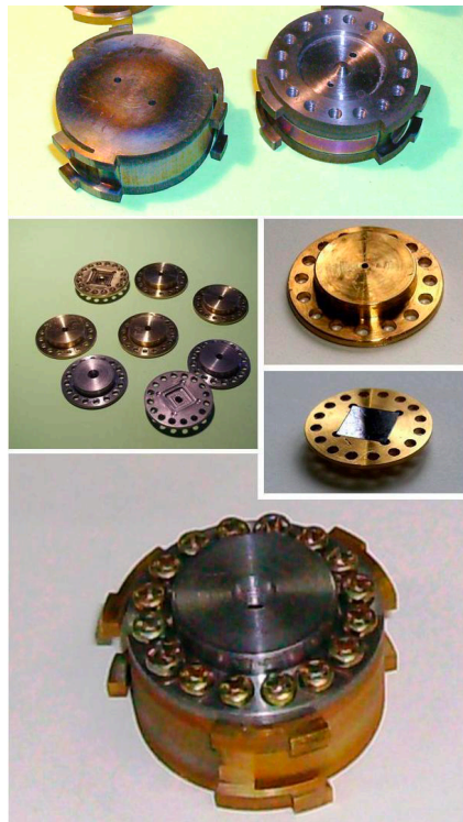
Figure 3. (Top and middle) Various views of the parts of the second designed transducer; (Bottom) The second designed transducer assembled. We succeeded to achieve electrical Qs as high as 3 \times 10^5 with this design, but the coupling to the cavities depended on a transmission line of 2 cm, which was presenting construction problems. We decided to remove this transmission line, mounting the microstrip antennas on the same side as the microwave cavity.
