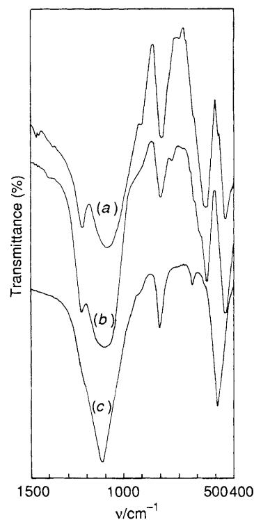
Fig. 2 IR spectra of (a) the original chromosilicate sample, (b) the sample treated with oxygen at 693 K, (c) the sample treated with oxygen at 843 K
