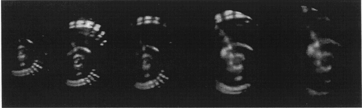
Fig. 5. Magnification at five positions of the second diffracting element.
