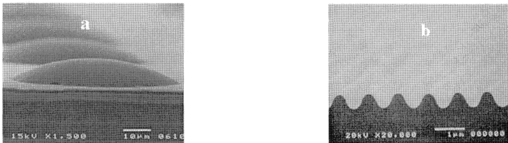
Figure 2: SEM microscopy showing a) the typical profile of a microlens master and b) the periodic relief structure of a DOE.
