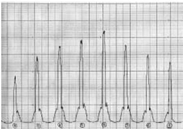
Figure 2. Intensity calibration curves of the 8 parallel spectral channels, 1 to 8, from right to left, of the multichannel detector XP 1752.
