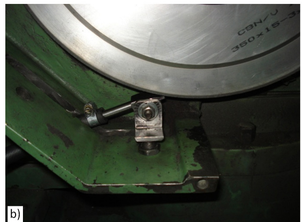
Figure 3. (a) Wheel cleaning nozzle design; (b) nozzle positioning ( 30^\circ in relation to normal angle).
