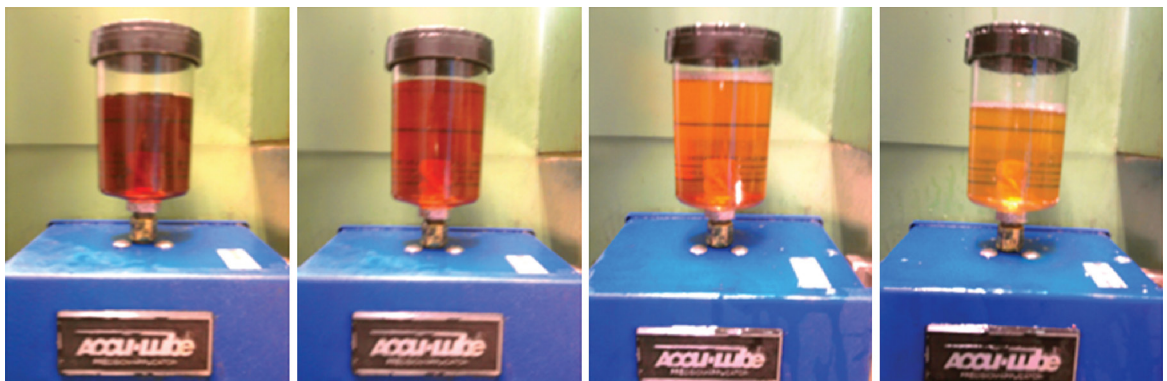
Figure 1. Cutting fluid dilution for MQL with water. From left to right: pure oil, 1:1, 1:3 and 1:5 parts of oil/parts of water.
