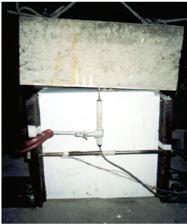
Figure 12 – Photo of typical rupture in the model without treatment of the column face with mortar containing additives
