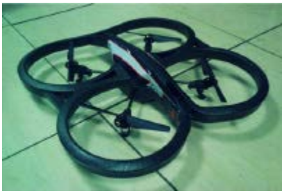
Figure 1. An AR.Drone quadcopter using indoor hull.
