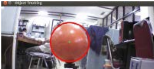
Figure 13. Object detected with distance of 0.5 meter.
