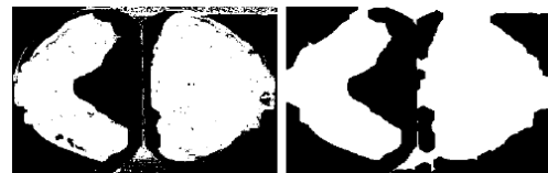
Figure 13. Example of resulted mask before (left) and after (right) noise reduction using morphological transformation.
