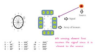
Fig 5. Representative diagram of Direction of Arrival sensor working
