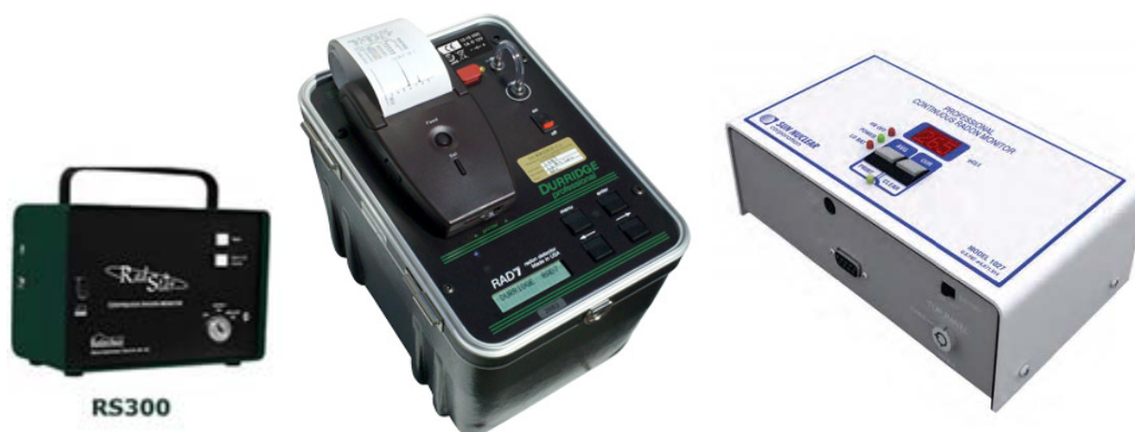
Figure 3.16: Examples of continuous radon monitors: RadStar Continuous Radon Monitor, RAD7, Sun Nuclear Model 1027
