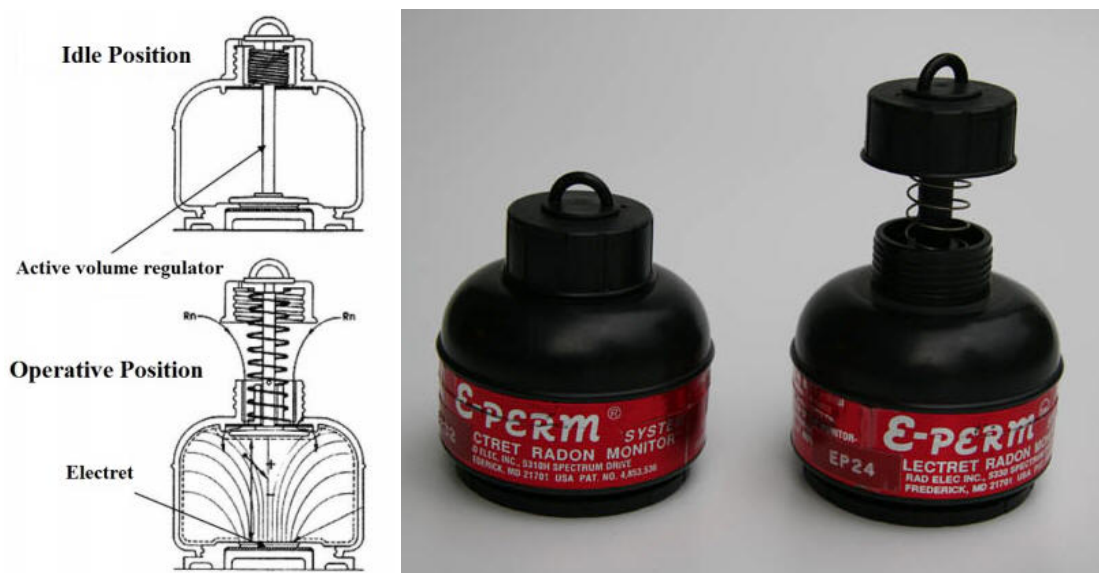
Figure 3.15: The electret ionization chamber. Scheme (left) and the appearance (right).
