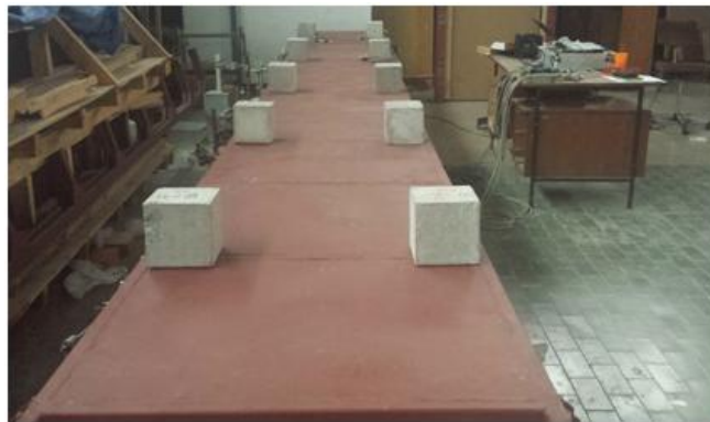
Figure 5.23: Grid-bridge model in the additional mass state
