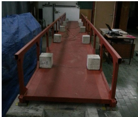
Figure 5.35: Masses distribution along the bridge deck for the model with additional mass state
