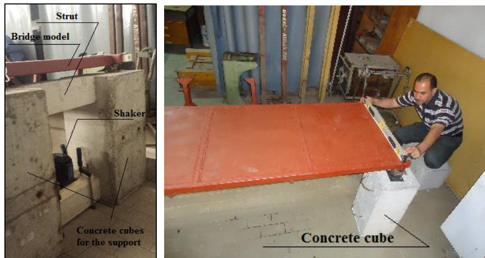
Figure 5.22: Grid-bridge model on concrete supports
