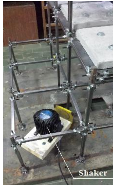
Figure 5.49: Installed shaker on the rigid steel base of the MSB model
