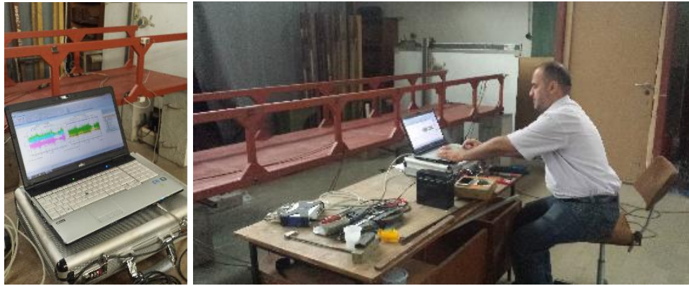
Figure 5.37: Vierendeel bridge model during AVM
