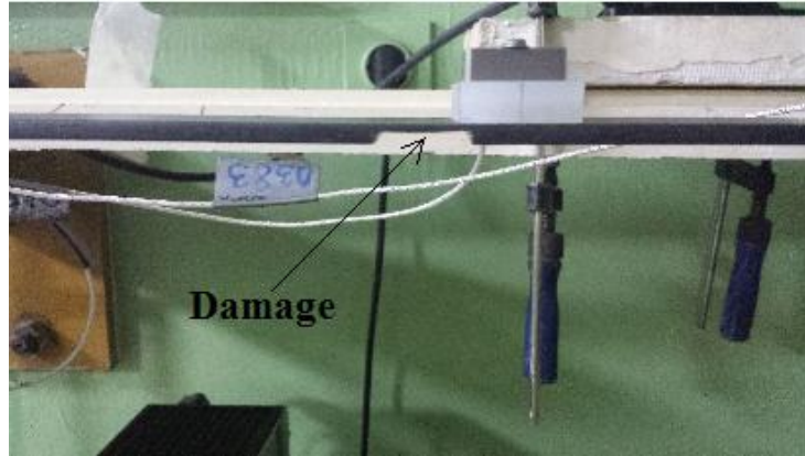
Figure 5.17: Reinstalling model for the test of second damage scenario
