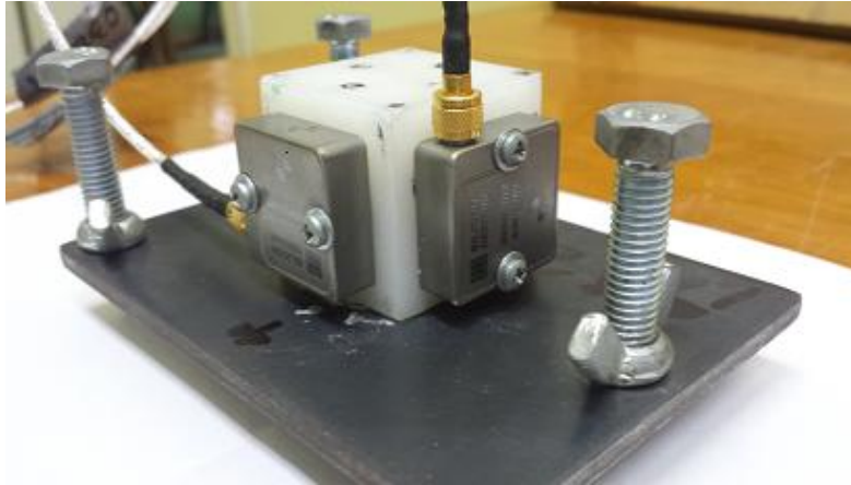
Figure 3.8: Installed accelerometers in two perpendicular directions of measurements
