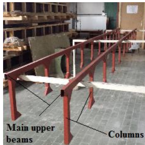
Figure 5.32: Fences of the Vierendeel bridge model
