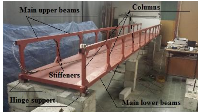
Figure 5.33: Vierendeel bridge model
