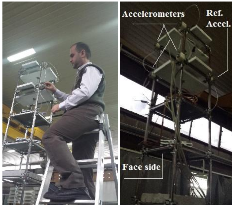
Figure 5.47: Installing of accelerometers on the tower part of the MSB model
